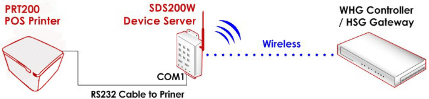
Diagram of SDS200W Connecting to PRT200 and WHG Controller wirelessly
